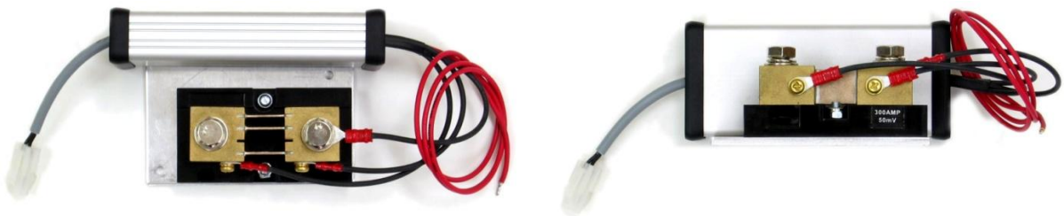
Figure 6: HV1/HV2 with shunt resistors
