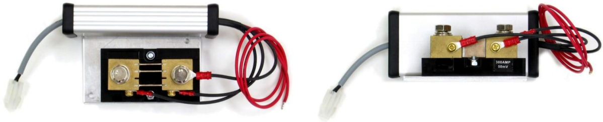
Figure 6: HV1/HV2 with shunt resistors
