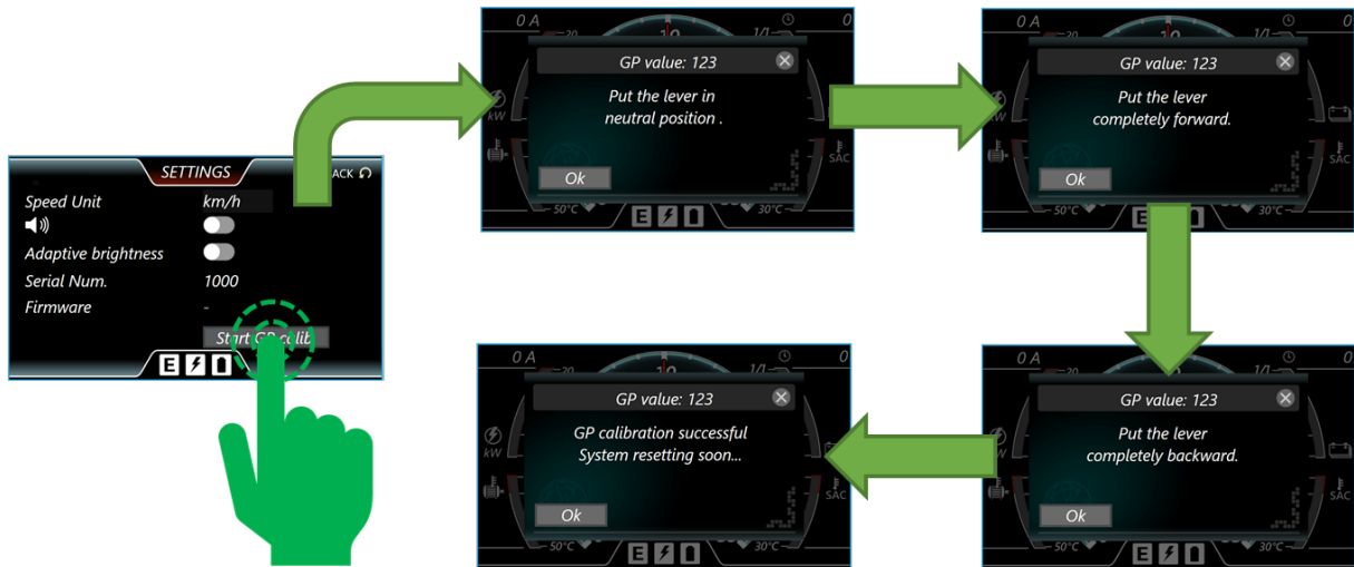
Calibration of the control lever - procedure
