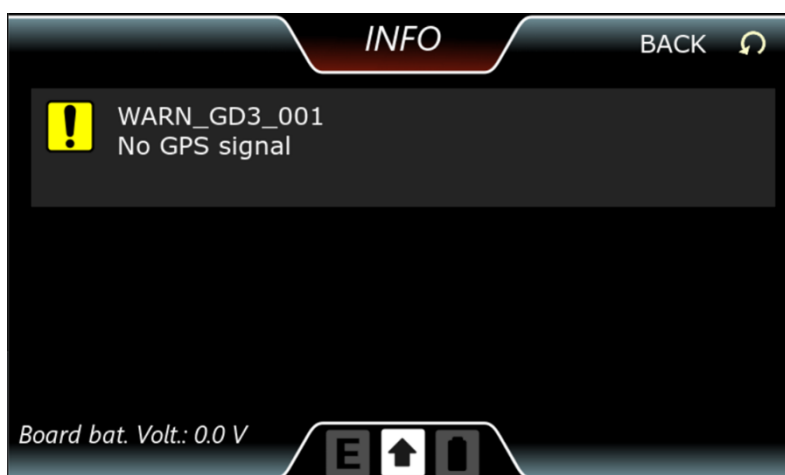
Error display in the case of missing GPS signal
